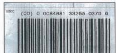
This example exhibits streaks at the top of the barcode and throughout the label.
